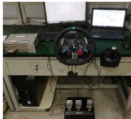
Fig. 19 Test platform of the driver model
